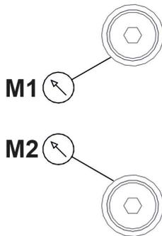
M1 and M2 connectors are pneumatic inputs used for external capillary connection (option).
