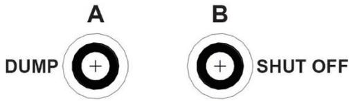
DUMP: pneumatic output to connect to an external valve for dump option.
