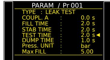
2. Use the up/down up/down keys to modify the parameter value, and press **OK** to validate.
