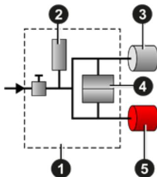
The part under test **3** and the reference part **5** are filled to an identical pressure.
