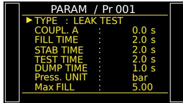
Default parameters of the type tests
