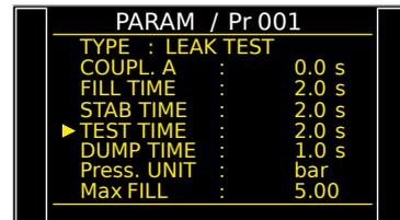
An arrow is displayed on the right of the parameter being modified.
