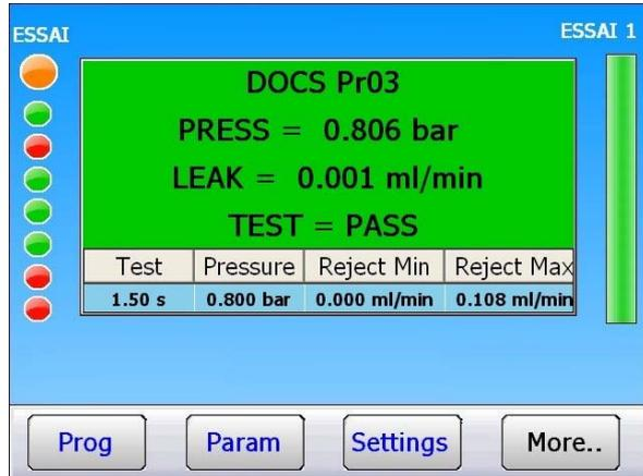
Used to display measurements and adjustable parameters.
