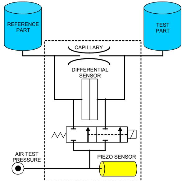
With this kind of instrument it is very important to have a reference volume, with if possible the same volume to the test part (the ideal thing is to have to same parts).
