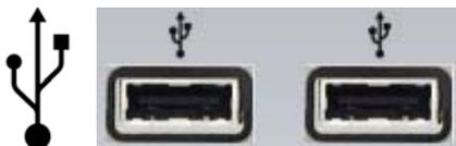
Allows the connection of various elements **USB** compatible (mouse, keyboard, memory etc.).
