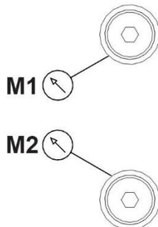
M1 and M2 connectors are pneumatic inputs used for external capillary connection (option).
