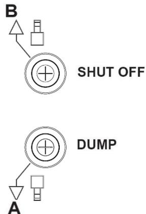
DUMP: pneumatic output to connect to an external valve for dump option.
