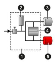
The part under test 3 and the reference part 5 are filled to an identical pressure. A differential sensor 4 measures the pressure variation between the part under test 3 and the reference part 5. In some applications, the reference part can be replaced by a cap.
