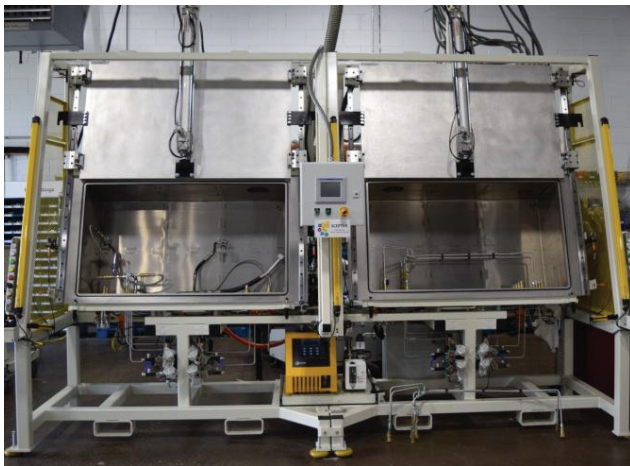
A standardized solution for thermal leak testing equipment. The Scepter is offered as a single, dual or IHX configuration
