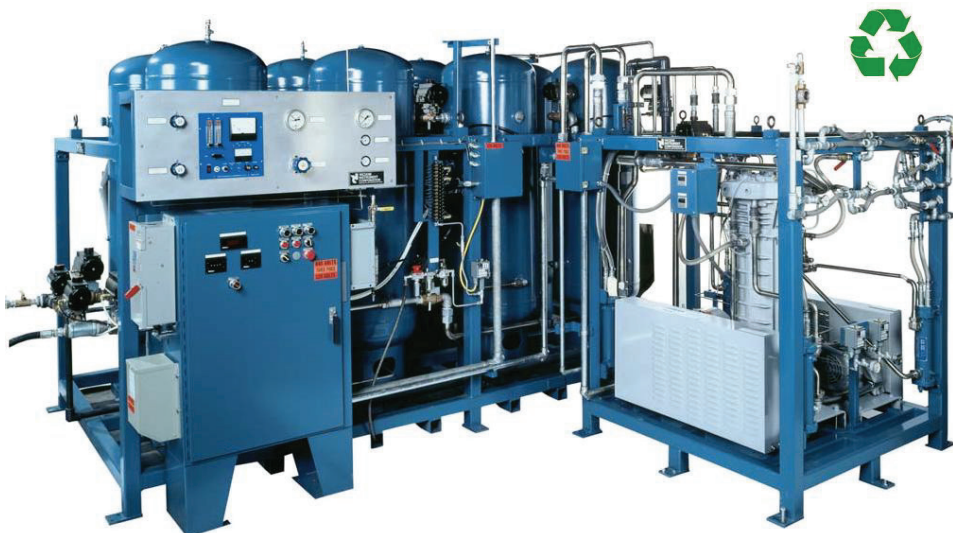
24 SCFM Recovery System
